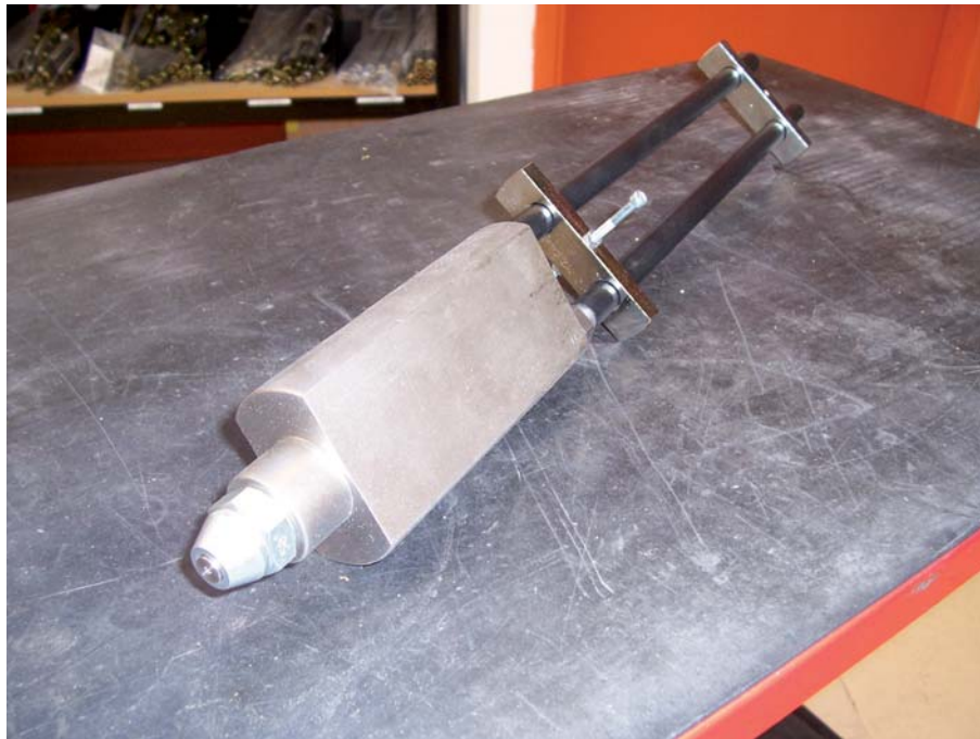
Oil nozzle and lance assembly
